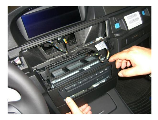
Steps 4-6 **4. Remove the 4 screws shown in the picture. Then pull Multimedia unit out. Be careful not to scratch the gear shifter (use towel).**
